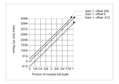
Analog X, Y, and Z Applying calculated gains to analog input
