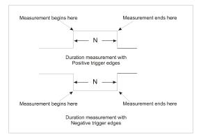
Time n is collected. Only the first pulse is measured. It must be reset to measure another pulse.
