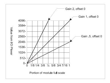
Applying both calculated gains and offsets to analog inputs simultaneously
