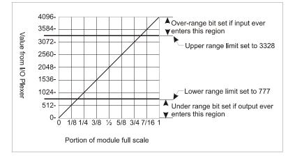
This instruction may be used for triggering alarms or capturing data where response needs to be faster than the host to I/O Plexer network serial link can react. Using this feature, very fast events can be recorded for the host to review after the event has occurred. The reaction speed of the I/O Plexer varies depending upon the number of analog input channels installed in the system.
